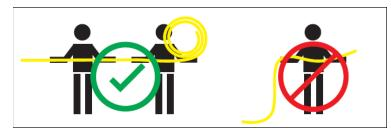
Only bend the neon in its intended direction. Do not twist or stretch neon. Above image shows horizontal bending neon.
