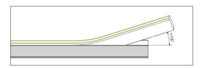
Align the neon with the channel and smoothly press it into place with your palm to avoid applying pressure to a single point. Keep the angle between the neon and the channel to less than 15-degrees to avoid bending it in the wrong direction.
